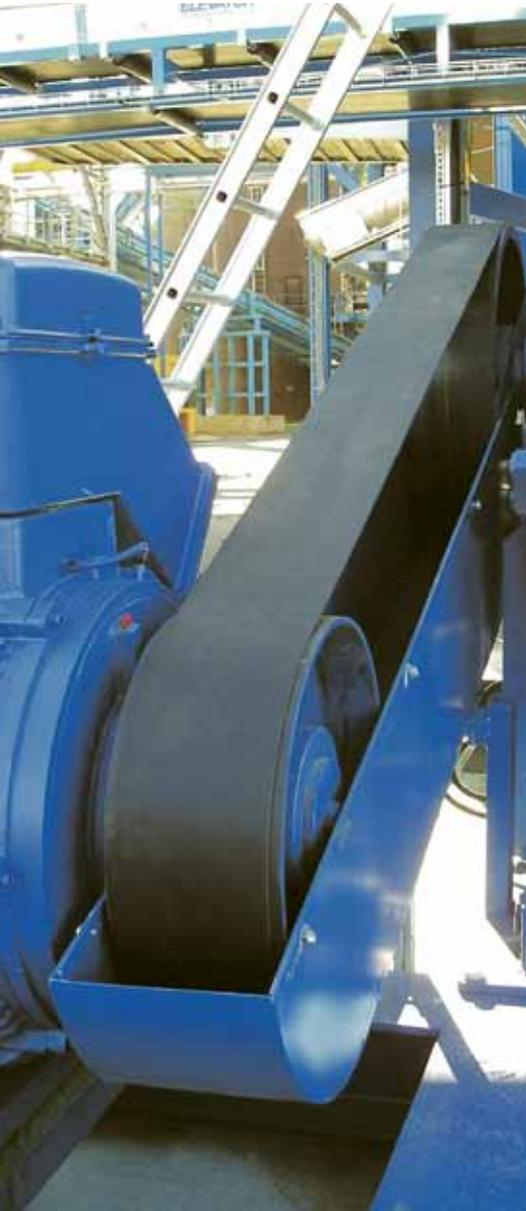
**Siegling Extremultus belts excel at transmitting vast amounts of power proficiently. They are extremely efficient and often a welcome alternative to high-loss gear boxes.**
