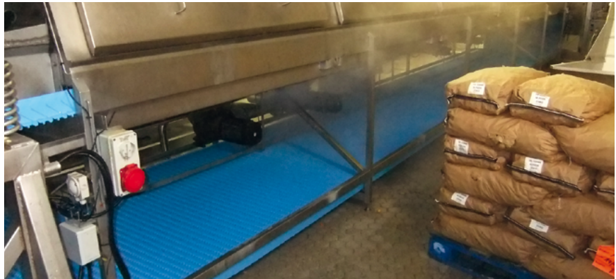
Forbo Siegling swapped the belt, reinforced with steel loops, for a much lighter modular one.
