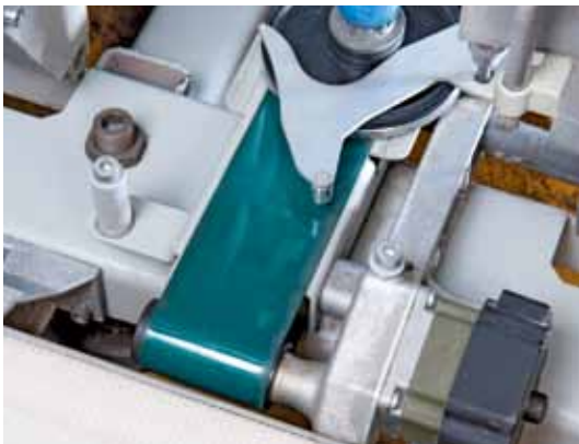
Ring spinning machine (four spindle drive)
