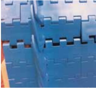
1 Move both belt ends until they interlink correctly
