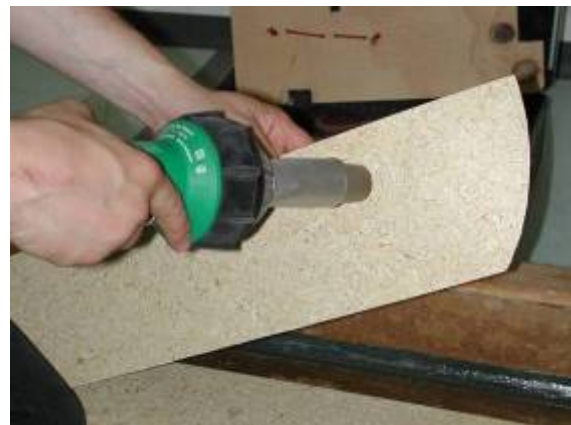
...and warm up with the hot air gun to bend.
