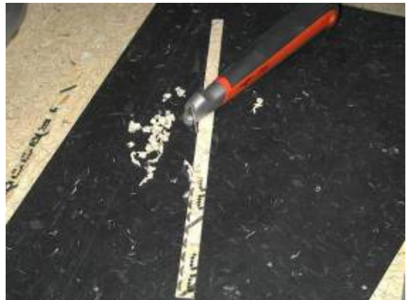
Scrap the Unigrid off the back with a scraper
