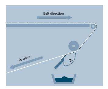
Fig. 1: Example of a belt scraper's position on the underside at an angle (A) of approx. 100°.
