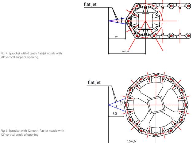
Fig. 5: Sprocket with 12 teeth, flat-jet nozzle with 42° vertical angle of opening.
