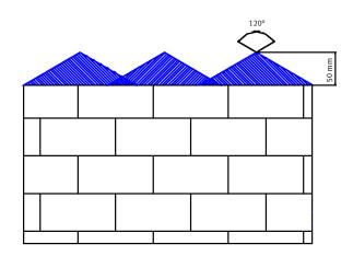
Fig. 3: Example of a nozzle layout with a horizontal opening angle of 120°.
