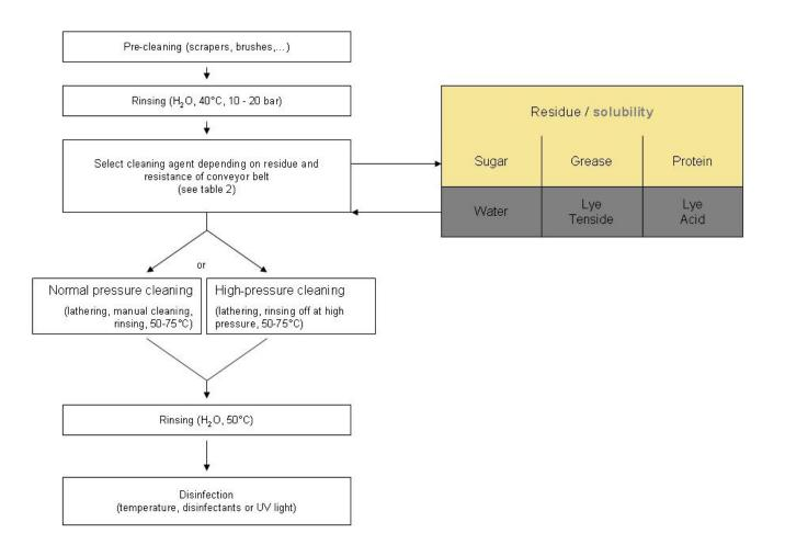
Fig. 2: Procedure for cleaning a conveyor belt in the food industry.
