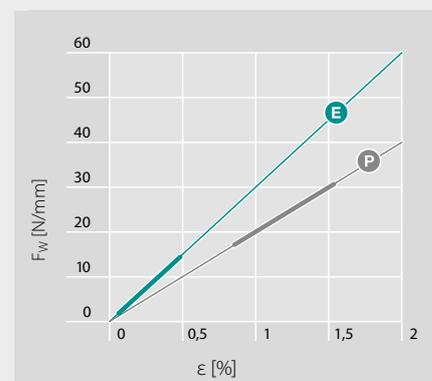
Thanks to the low elongation at fitting (area marked) the Polyester types produce a lower shaft load in comparison to conventional products with polyamide tension members.
